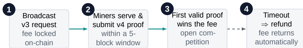
Figure 2: Lifecycle of an on-chain inference request. If no valid proof arrives within the confirmation window, the locked fee is returned to the sender automatically.
